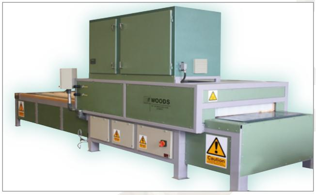
The WOODS range of RF laminators can greatly enhance the production of staircase components. The practical design and operational simplicity of the laminators make them an ideal tool for bonding the many diverse components used in staircase manufacturing, in both hardwood and softwood.
